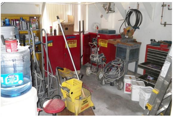
Photo No. 14 Paint sprayers, various hand and power tools, and three metal cabinets labeled "flammable" containing retail-size containers of paint thinners and aerosol paints in the paint shop
