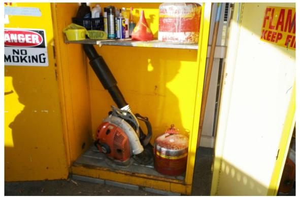
Photo No. 17 5-gallon containers of gasoline, leaf-blowers, and retail-size containers of lubricant in the metal storage cabinets in the equipment storage enclosure
